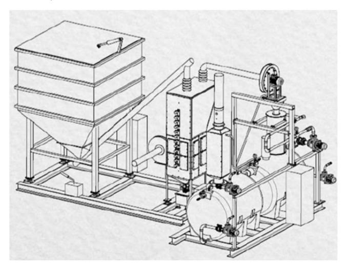
The **first tests** put in evidence some empirical complications related to the insufficient cochlea speed, choking problems caused by manure inside cochlea, difficulties in hopper loading and ashes flow problems. However, 3P engineers overcame all those, below is explained how.
